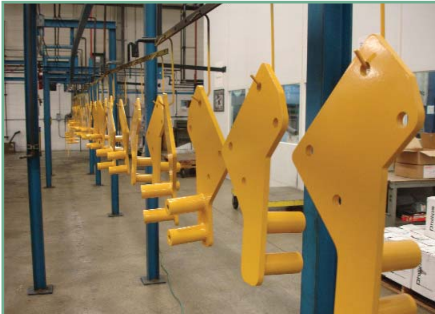
Figure 4: Professional Plating's powder coating line features a 10-stage pretreatment process with iron phosphate and non-chrome sealant.
