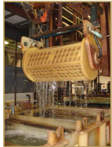
Figure 3: This 13-barrel, 22-station plating line allows Professional Plating the ability to process thousands of pounds of material daily.
