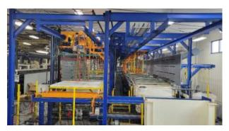
This is our third rack zinc line. It is slightly smaller than our existing two rack zinc lines. Rack 6 can plate parts 12" wide x 6' in length.
